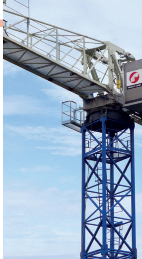
City Lifting erected a special version of the Linden Comansa 21LC750 flat top tower crane for work at London's Heathrow Airport
